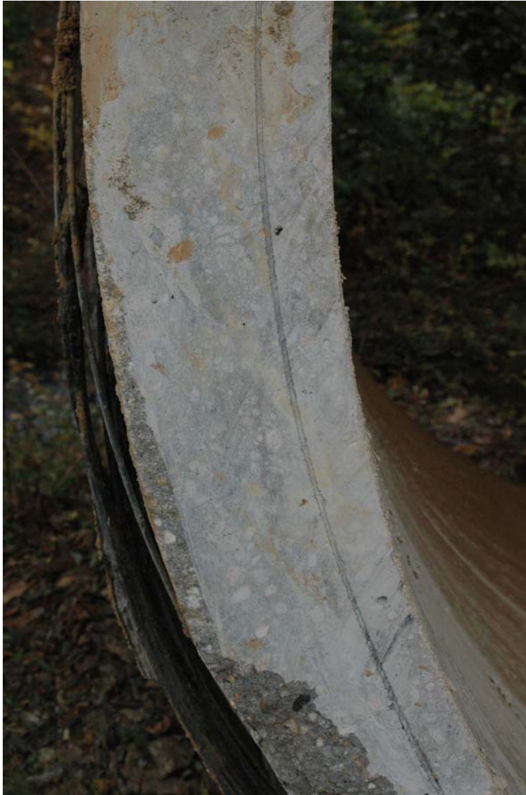
Cross section of pipe wall
