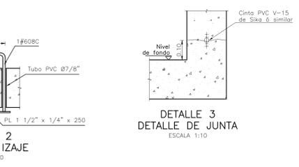
DETALLE 3 DETALLE DE JUNTA
